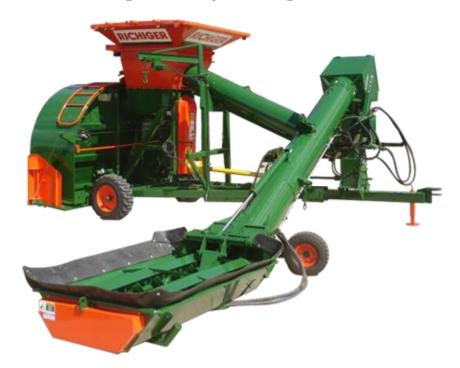
The CG300 combines hydraulic and mechanical drives to achieve high capacity unloading. This will load 9 or 10ft baggers, using a 100HP tractor. The transfer auger sets up for work in minutes. Its 180 degree foldaway hopper results in shorter lengths than competitors machines for better maneuverability in the yard and on the road.
