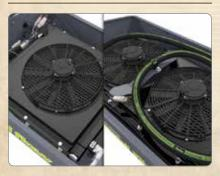
High Capacity Cooling: The single-fan model offers an impressive 95,000 BTUs per hour of cooling capacity for mid-frame skid steers. The twin-fan Cool Flow offers industry-leading cooling performance for extreme temperatures and job applications with 140,000 BTUs per hour.
