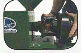
RTU-1250LP drive being disconnected from the R950, R1050 or R950MX bagger
