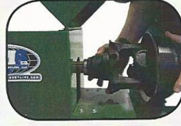
RTU-1250LP drive being disconnected from the R950, R1050 or R950MX bagger
